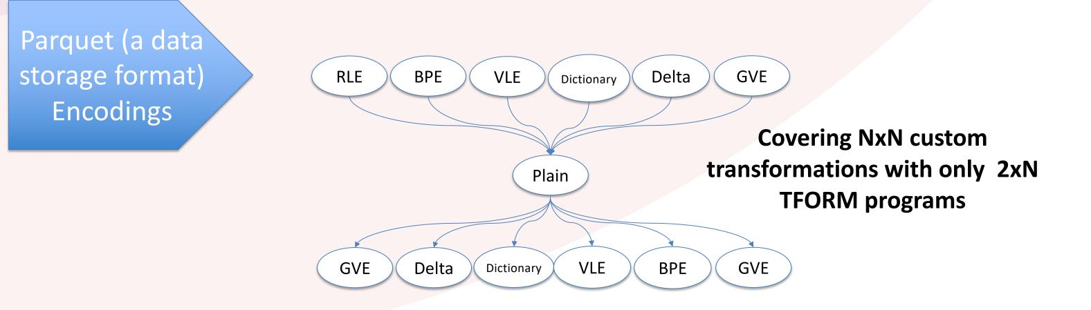
• We use TFORM programs for efficient data transformation on CPU, Unstructured Data Processor (UDP) [1] (a general data transformation accelerator), and UpDown Engine [2] (a memory-movement and recode accelerator embedded in memory
