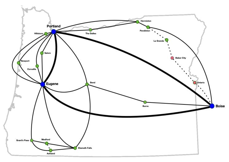
Each circuit is DWDM lambda terminated as a 2x100GBase Ethernet LACP bond
