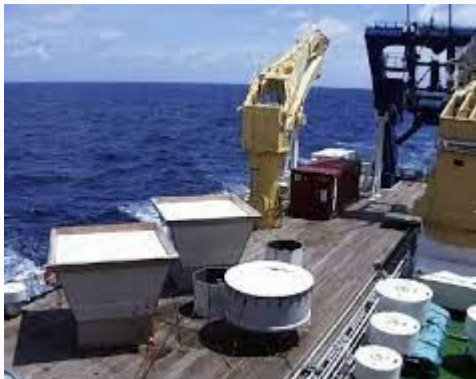
Two wind profiler radars (large white boxes) on the deck of the R/V Menai. One is a 300W and the other is a 100W. There is also a RASS system and an S-band vertically pointing radar (the arm at the end).
