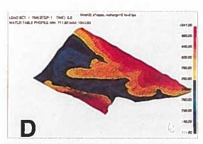
Computed Water Table Elevations after Capping
