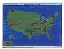
The NASA Aeronautics Network (AERONet) provides computer networking facilities to the aerospace community. NASA centers are linked via high speed communications lines, and lower-speed tail circuits connect other members of the aerospace community to NASA. In addition, AERONet also provides Internet access with many other networks, thereby increasing national and international network connectivity.
