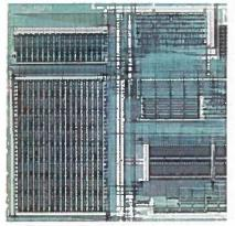
NIST's MultiKron chip provides low perturbation measurements for performance evaluation of computer and communication systems.
