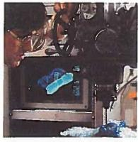
A machinist monitors a machine tool retrofitted with a personal computer controller. The machine is located in NIST's Shop of the 90s where manufacturers can learn how to use open system integration technology and low-cost automation techniques to improve productivity and product quality.
