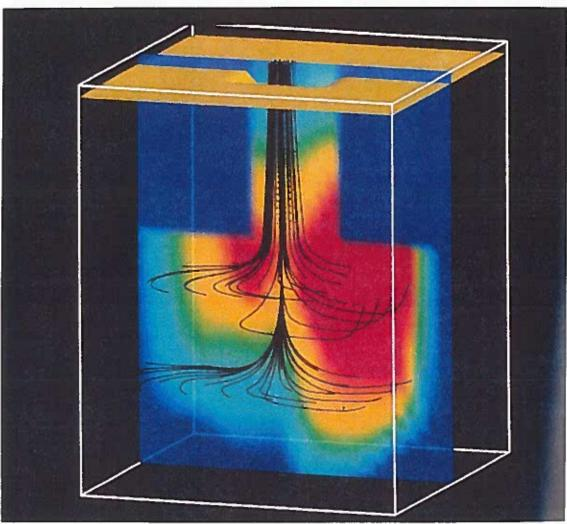
The results of applying a fully-scalable parallel iterative matrix solver to create a three-dimensional simulation of current flow in a bipolar transistor are shown. The transistor was simulated on the Intel Delta at Caltech using software developed at Stanford University. This simulation is the largest yet in this field and represents the state of the art in three-dimensional device modeling. Such modeling efforts enable process design in the "Virtual Factory."
