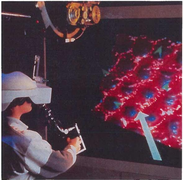
The photograph shows an investigator, with a head-mounted display and a force-feedback manipulator controlling the tip of a scanning tunneling microscope (STM) probe, exploring the surface of a sample of material. The image projected on the wall indicates the view that the investigator sees and changes as his head position and orientation change. The region of the surface shown is 25 Angstroms on a side.
