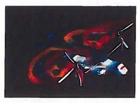
Simulation of a tiltrotor aircraft (V-22 Osprey) during takeoff. Shown are streaklines, rendered as smoke and computed using UFAT (Unsteady Flow Analysis Toolkit), a new time-dependent particle tracing code.
